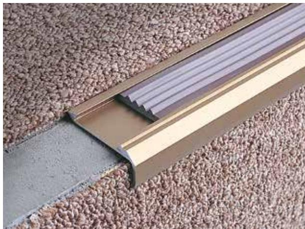
Aluminum and brass STAIRTEC SM stair nosing profiles are equipped with a non-slip, smooth or grooved rubber insert providing an ideal solution for staircases covered with thin floor types such as carpet and vinyl. The profile is installed with flathead screws placed under the rubber insert.
